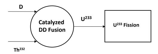
Material flows in the DT (top) and Catalyzed DD fusion-fission hybrid (bottom) Fuel Factory alternatives with U<sup>233</sup> breeding from Th<sup>232</sup>.
