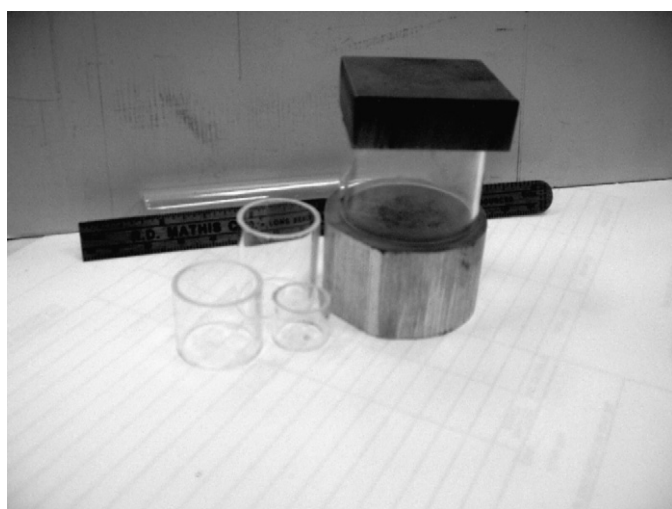
Fig. 1. Glass cylinders used in several boron depositions. The tube between the metallic plates/electrodes placed in vacuum creates a deposition capacitor.
