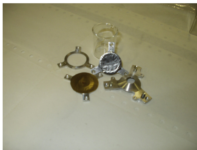
Fig. 2. Frames with foil ready for a stretching test on a conical-shaped Al base.
