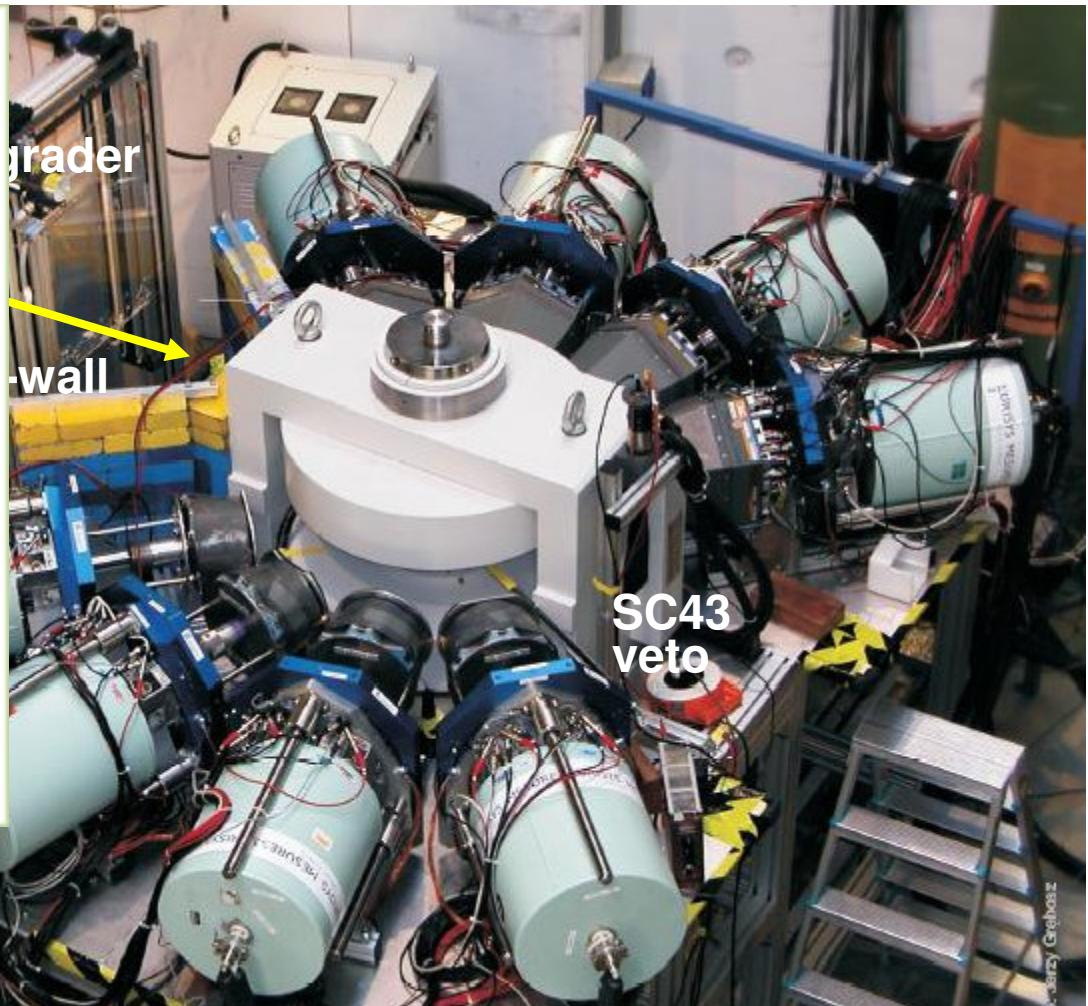
4 clusters with BGO anticompton shields and short collimators
