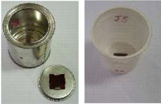
Figure II.6. Photo of two types of diffusion chambers used for practical investigations (left – metal chamber, right plastic chamber). The SSNTDs in both are Kodak Pathe LR-115 type II films.
