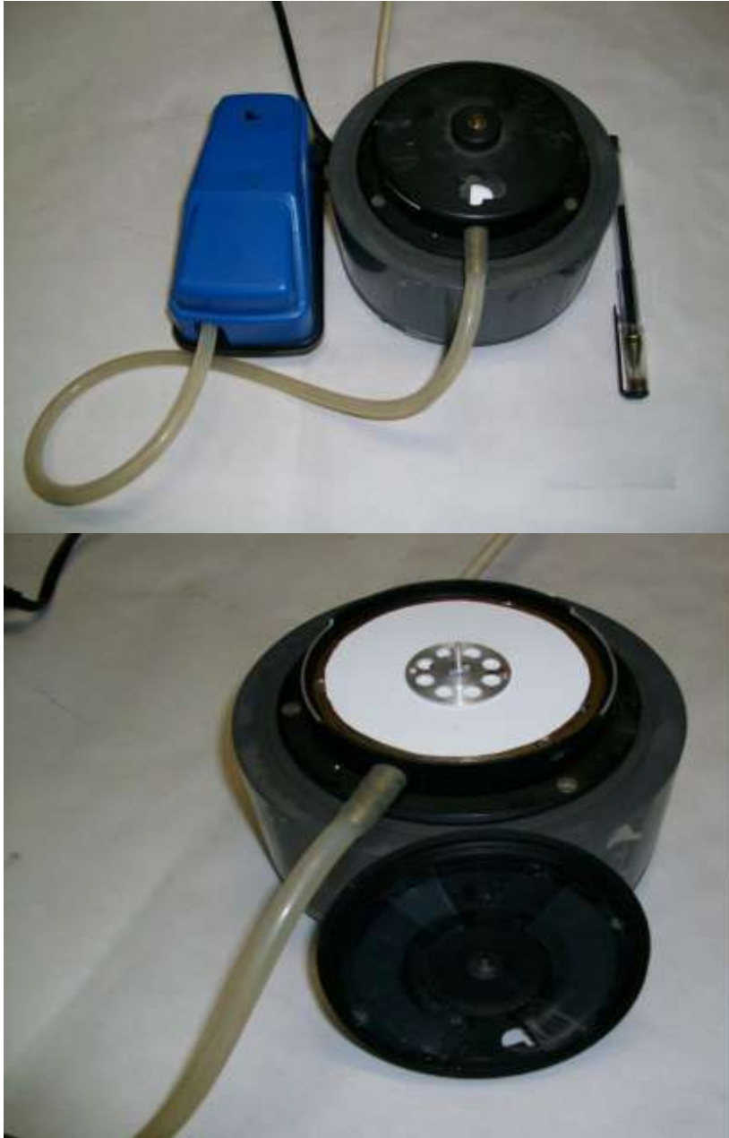
Figure III.2. A photo of the experimental device. Above: the device ready for use; below: The filter and the cap with SSNTD film covered with Mylar absorber foils.
