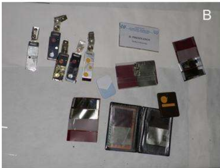
Figure VII.11. (A) Photo of empty badges and envelopes, used in experiments. (B) Badges and envelopes with radon films inside. In each package a SSNTD with M-absorber and/or C-absorber is placed – in some cases several different absorbers are used.
